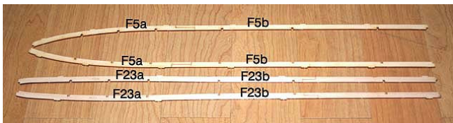
2. Glue the longerons(F5a-F5b, F23a-F23b) together.
