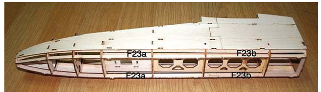
8. Assemble and glue longerons(F23a,F23b) with thick CA .
