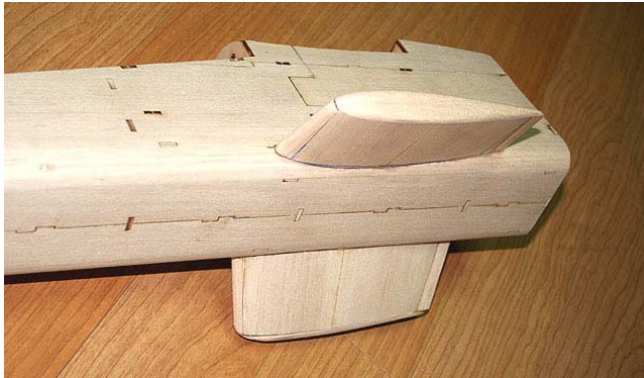
5. Glue sponson to the fuselage with thick CA .
