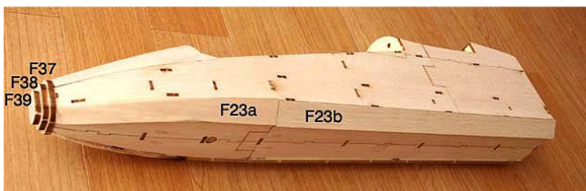
13. Glue edges(F23a,F23b) and nose cones(F37-F39) with thick CA .
