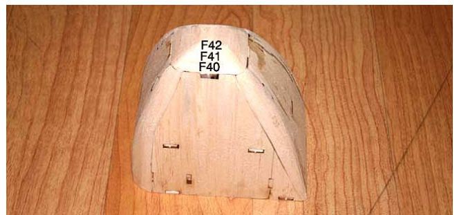
18. Glue and rear cone(F40-F42) with thick CA . Carefully sand surfaces.
