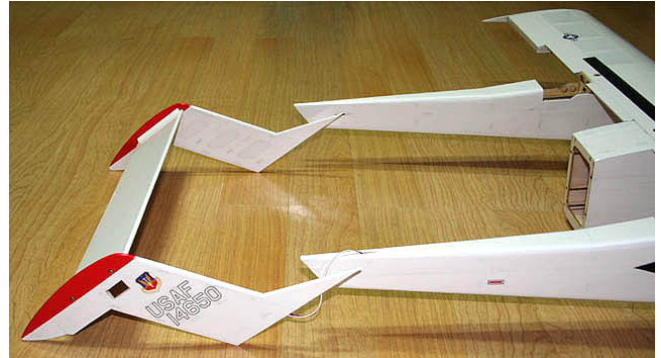
2. Assemble tail and insert elevator servo extension.
