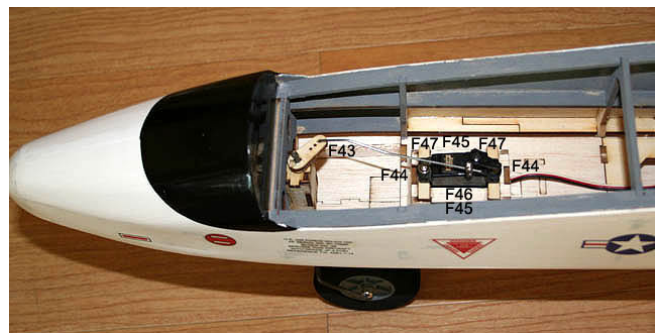
14. Install nose gear and fix with wheel collar below and above of mount. (Optional) Assemble and glue nose steering servo mount (F44-F47) and install nose steering arm, drill, tap and fix to the collar with small bolt.
