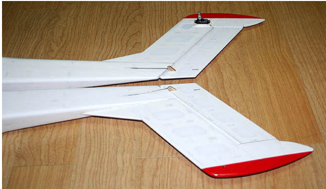
8. Insert rudder pushrods to the horns and then glue hinges to the fin with small amount of thin CA.
