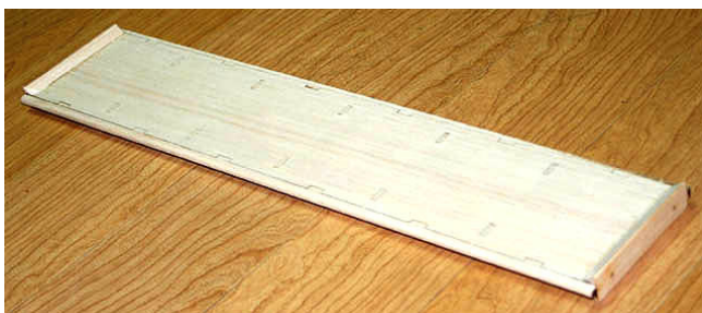
7. Sand H9 parts as shown above.
