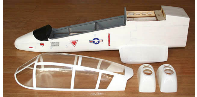
12. Paint canopy, cowl and cockpit area.
