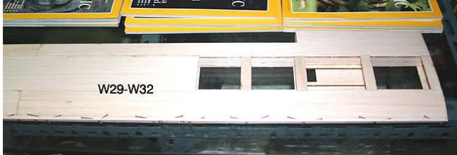
9. Cover the top sheet(W29-32). Hold down the front edge with pins to the sub leading edge.
