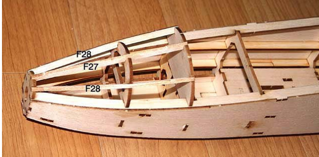
10. Assemble and glue longerons(F27-F28) with thick CA .
