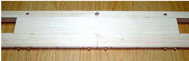
11. Insert wing dowels and glue.
