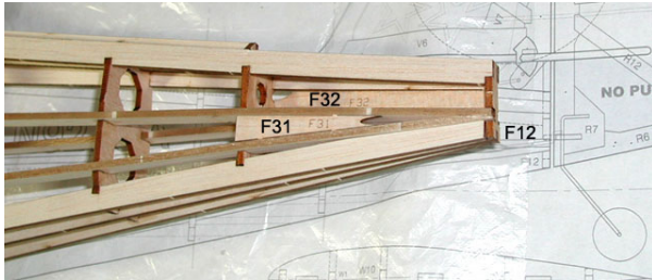
17. Glue bulkhead(F12) and panels for pushrod exit(F31, F32).
