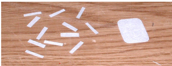
4. Cut CA hinges as shown above.
