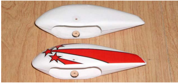
17. Glue Plywood rings with thin CA and put color stickers on.
