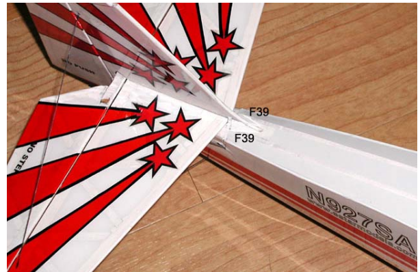
22. Paint or cover film after shape and glue F39 parts.
