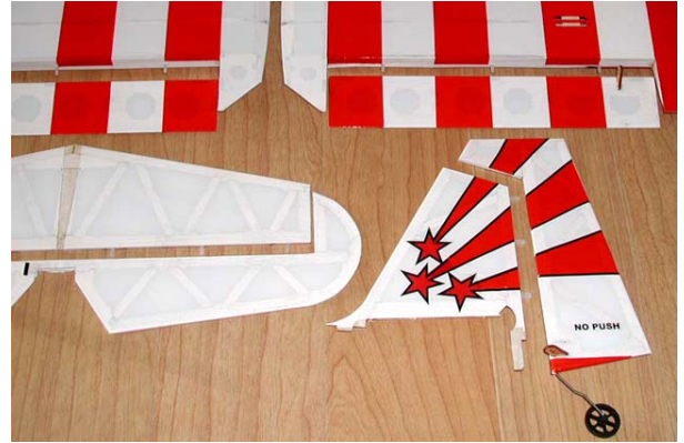
5. Install and glue aileron and rudder plywood horns. (Do not glue elevator horn in this step.)
