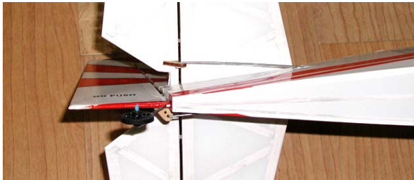
9. Glue stabilizer and vertical fin to the fuselage with thick CA. (Horizontal tail must be paralleled with wing and vertical fin must be at right angle to horizontal tail. Wings must be installed temporarily to align them.) Insert elevator pushrod to the horn and then glue hinges with small amount of thin CA. Insert rudder pushrod to the horn and then glue hinges with small amount of thin CA.
