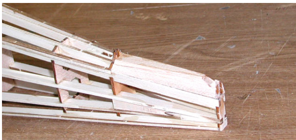
21. Shape and sand stabilizer bed.
