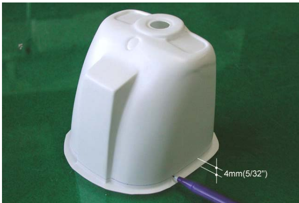
20. Draw cutting line (4mm above from the bottom) and cut cowl.
