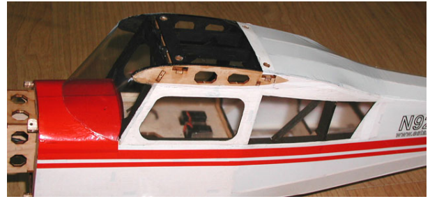
12. Cut clear plastic windshield and glue.(refer to template on the drawing). Cover side windows with clear film.
