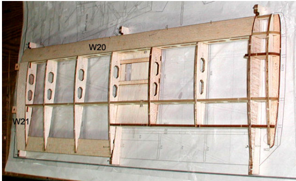
6. Glue upper sheets(W20, W21) with thick CA .
