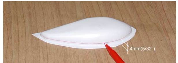
14. Draw cutting line. (4mm above from the bottom)
