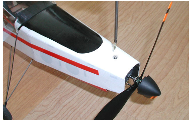
17. Install motor and fix with screw.
