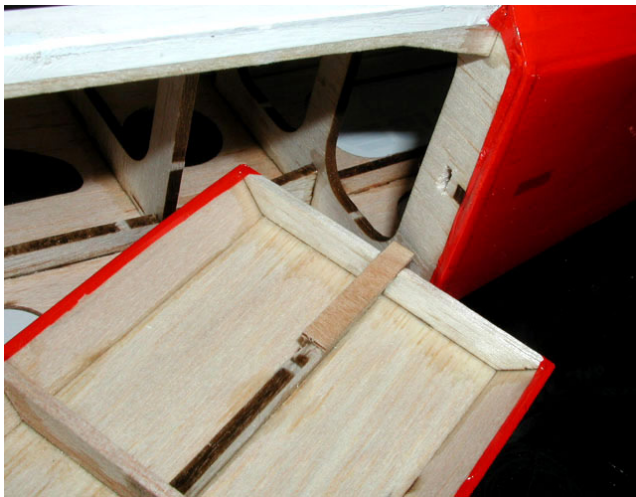
2. Glue the plywood dowel of hatch(H5).
