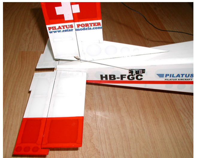
14. Install rudder servo and insert pushrods.
