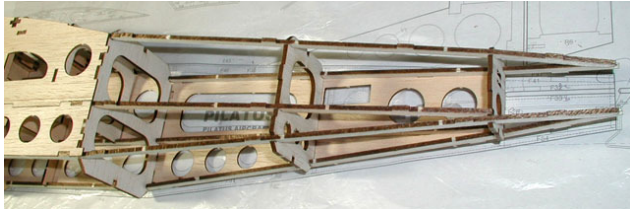
12. Temporary assemble rear longerons(F27-F28).
