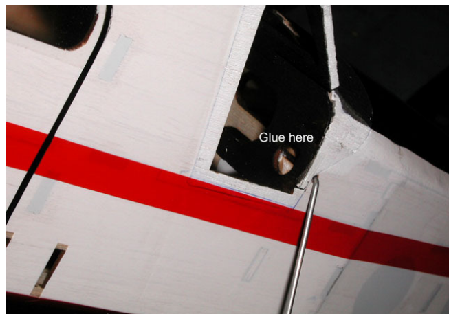
7. Install landing gear and apply thick CA.
