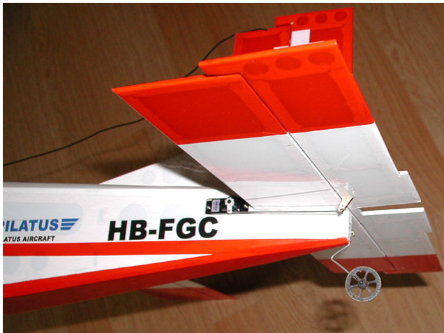
15. Install elevator servo and insert pushrods. Fix tail gear. (Use scrap of clear plastic.)
