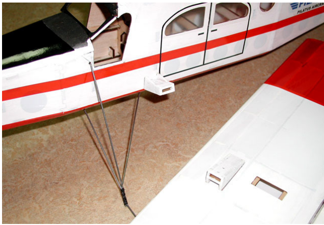
9. Insert and glue strut mounts.
