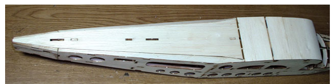
19. After sanding glue rear fuselage top cover(F45).
