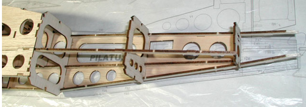
11. Temporary assemble rear right side panel(F37), rear longerons(F27-F28) and bulkheads(F29-F30).
