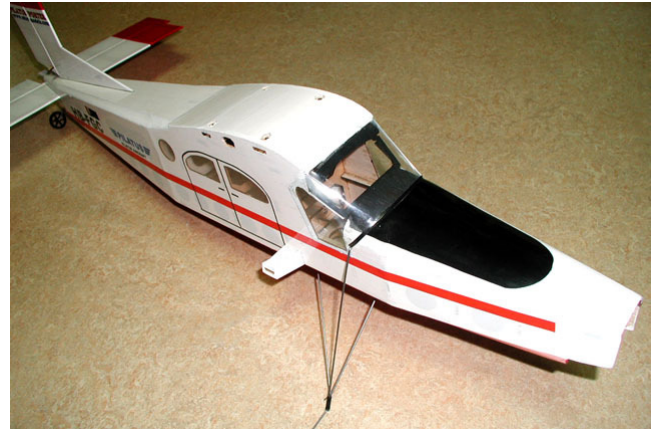
13. Cut clear plastic windshield and glue it.(refer to template on the drawing). Cover side windows with clear film.
