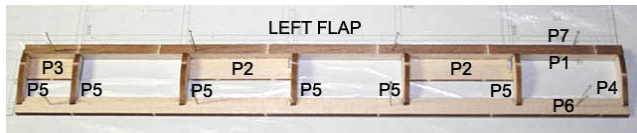
3. Pin the left flap parts(P1-P7) on the plan and glue together with thick CA.
