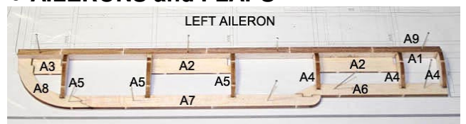
1. Pin the left aileron parts(A1-A9) on the plan and glue together with thick CA.
