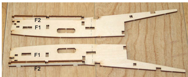
2. Assemble and glue the parts(F1, F2) with thick CA.
