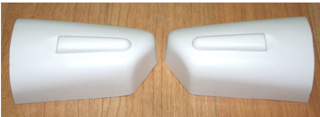
29. Cut cowl and carefully sand edges.
