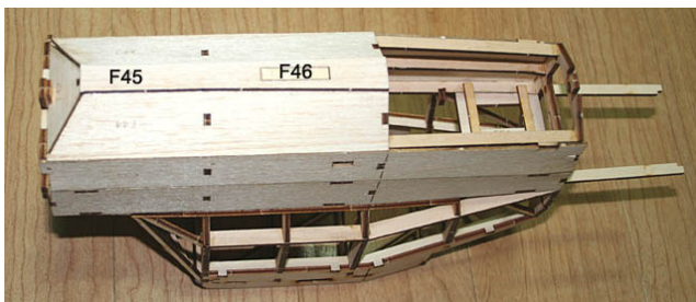
18. Sand part F44 and then glue the parts(F45-F46) with thick CA.
