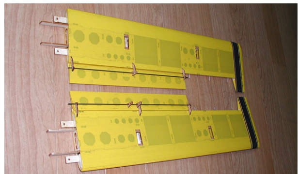
4. Insert flap hinges and horns(P8-P10). Use 2mm wire to align easier. Temporarily glue with small amount of CA. After throwing check, and then glue them firmly.
