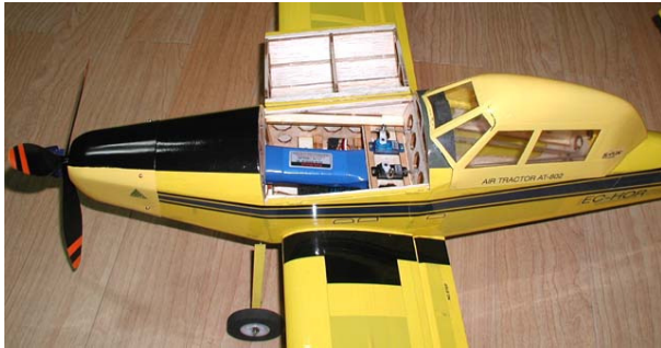
14. Fix cowl with screws and fix battery with Velcro tape.
