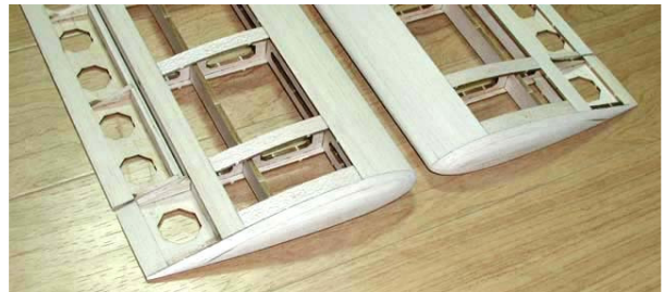
18. Carefully sand surfaces.
