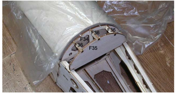
24. Temporary assemble hatch and then glue bulkhead(F34, F35) and longerones(F36) with thick CA . Use PVC film or waxed paper to prevent bonding with hatch.
