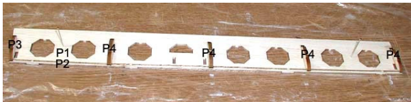
13. Assemble flap sub leading edge(P2) and ribs(P3, P4) and then, glue them.
