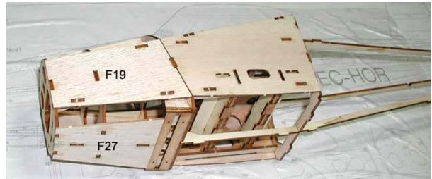
13. Assemble left side and bottom panel(F19, F27) and glue with thin CA.
