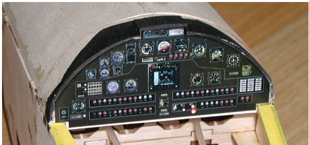
44. Attach instruments panel sticker.
