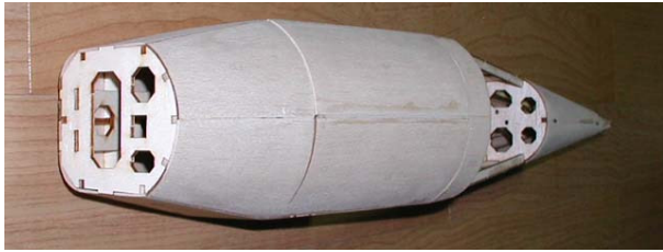
29. Carefully sand fuselage surfaces.
