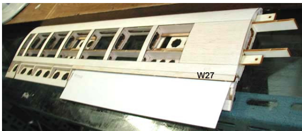
17. Glue trailing edge(W27) with thick CA . Refer to the wing section on the drawing and use cardboard to make a gap.
