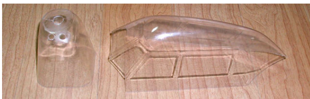
34. Cut cowl and canopy.
