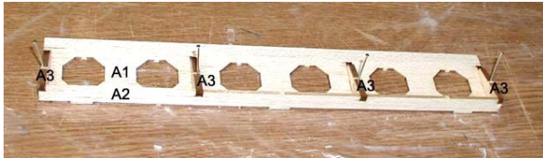
11. Assemble aileron sub leading edge(A2) and ribs(A3) and then, glue them.
