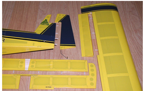
3. Make hinge slots and install hinges. (Do not glue hinges to the control surfaces in this step.)
