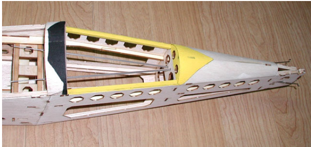
42. Insert and glue plastic pipes for elevator and rudder pushrods.
