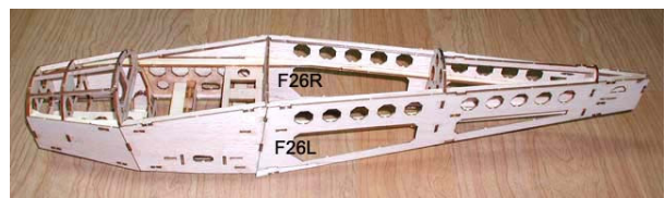
16. Assemble side panels and glue with thin CA. Apply thick CA glue at each joints for reinforcing.
