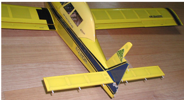
7. Glue stabilizer and vertical fin to the fuselage with thick CA . (Horizontal tail must be paralleled with wing and vertical fin must be at right angle to horizontal tail.)
