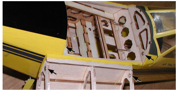
10. Install and glue neodymium magnetics with thin CA. Use scotch tape on the other side as a hinge of hatch.
