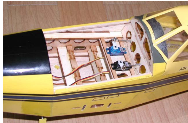
11. Install elevator and rudder servos.
