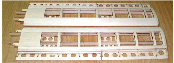
11. Assemble aileron sub leading edge(A2) and ribs(A3) and then, glue them.
