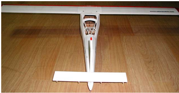
6. Glue stabilizer and vertical fin to the fuselage with thick CA. (Horizontal tail must be paralleled with wing and vertical fin must be at right angle to horizontal tail. Wings must be installed temporarily to align them.)
