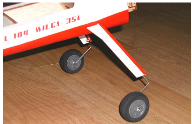
20. Install wheels to the landing gear.
