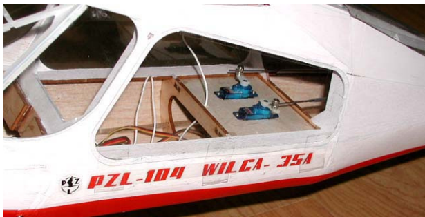
26. Cut clear plastic left side windshield, attach with clear tape. (This window should be a hatch for battery and your maintenance.)
