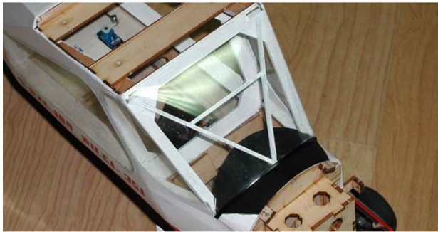
23. Cut clear plastic fore windshield, fold and glue.(refer to template on the drawing).
