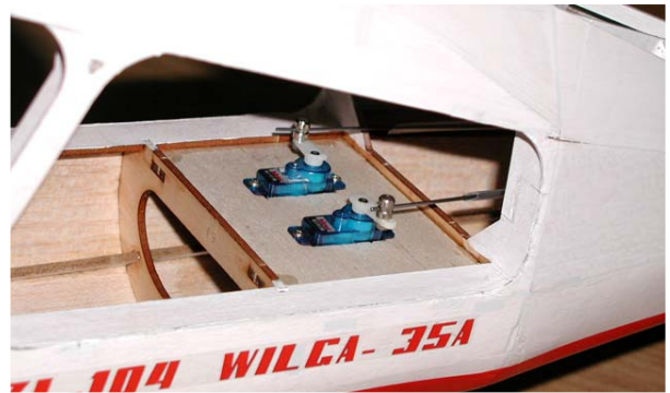
19. Install elevator and rudder servos.
