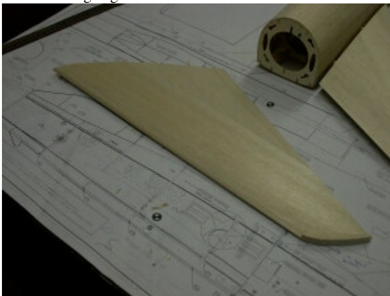
Glue and sand the 4x12x550mm balsa leading edge.
