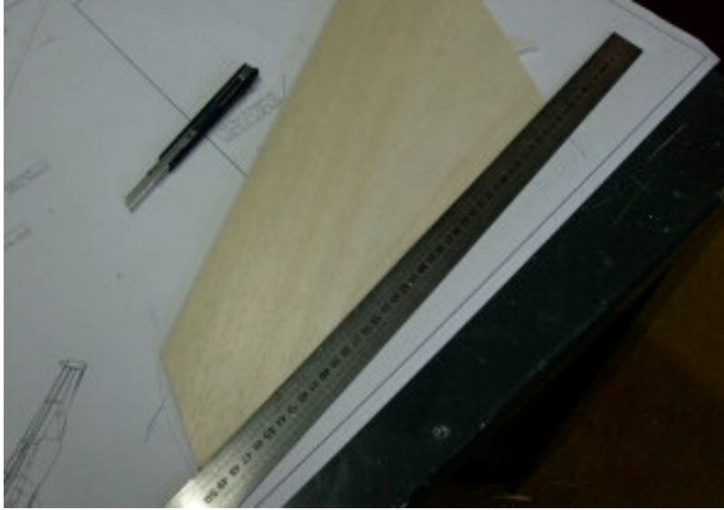
Cut and sand the wing panel to size.
