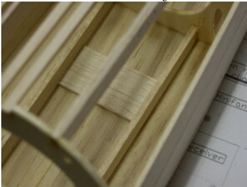
Glue a piece of 3mm balsa on the bottom for the servo's.
