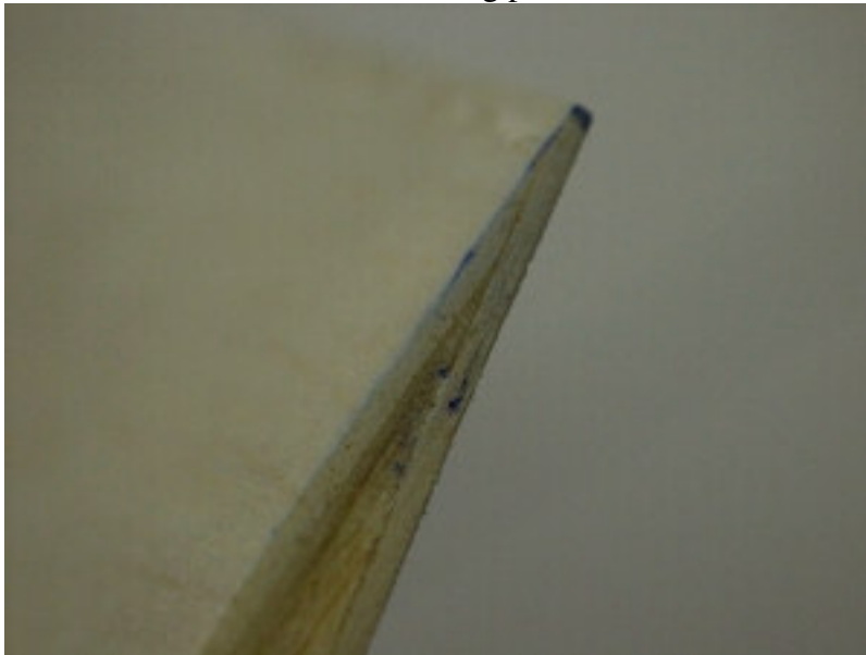
The trailing edge will look like this when sanded smooth.
