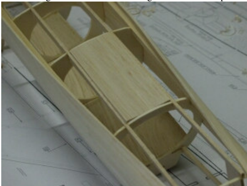
Glue the balsa sheet between F2 and F3 for the bungee hook.
