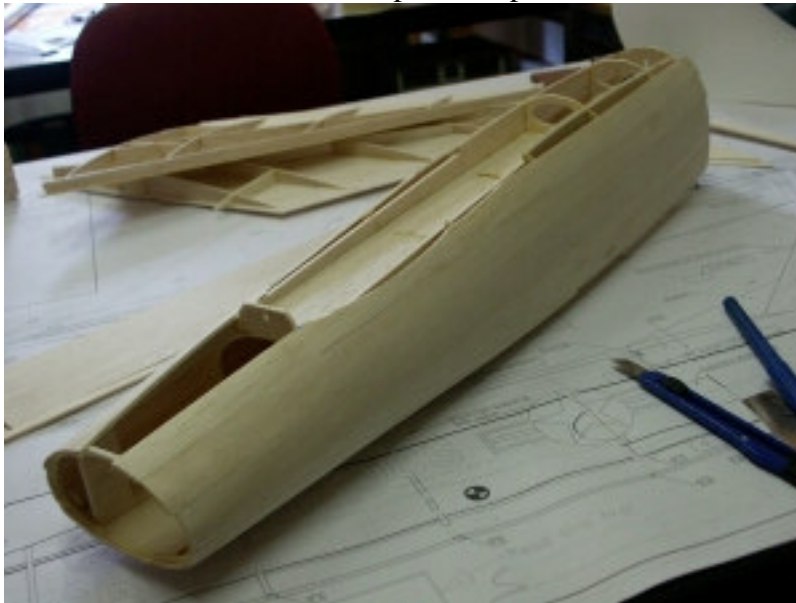
The top of the nose stays open that's that give good access when gluing the inlet tube.
